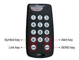
Power on keypad: Connecting keypad to base will initiate a two hours power on period.
